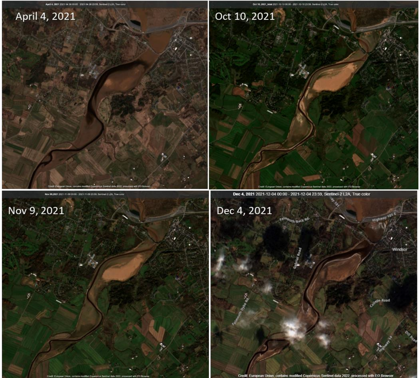
FIGURE 12: EVOLUTION OF TIDAL FLATS AND BEDFORM FEATURES UPSTREAM OF THE CAUSEWAY WITH GATES OPERATING ACCORDING TO MINISTERIAL MANDATE FOR FISH PASSAGE.
