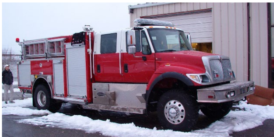
Engine 5 (South West Hants) – 2006 International 4 x 4 Engine. Has a 1050GPM pump and 625 gallon tank. Designed by Chief Fox for the Vaughan area. Crew Capacity of 5. 1 st out for any structure, vehicle fire etc.
