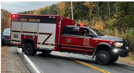
Rescue 5 (South West Hants) – 2020 Dodge 3500 4 x 4 rescue. Has a small pump and tank. Designed around brush fire response, with limited structural fire capability . Is not designed as a first in unit for this type of response. Carries an AMKUS electric combination tool (JAWS). Crew capacity of 5. 1 st out for medical calls.
