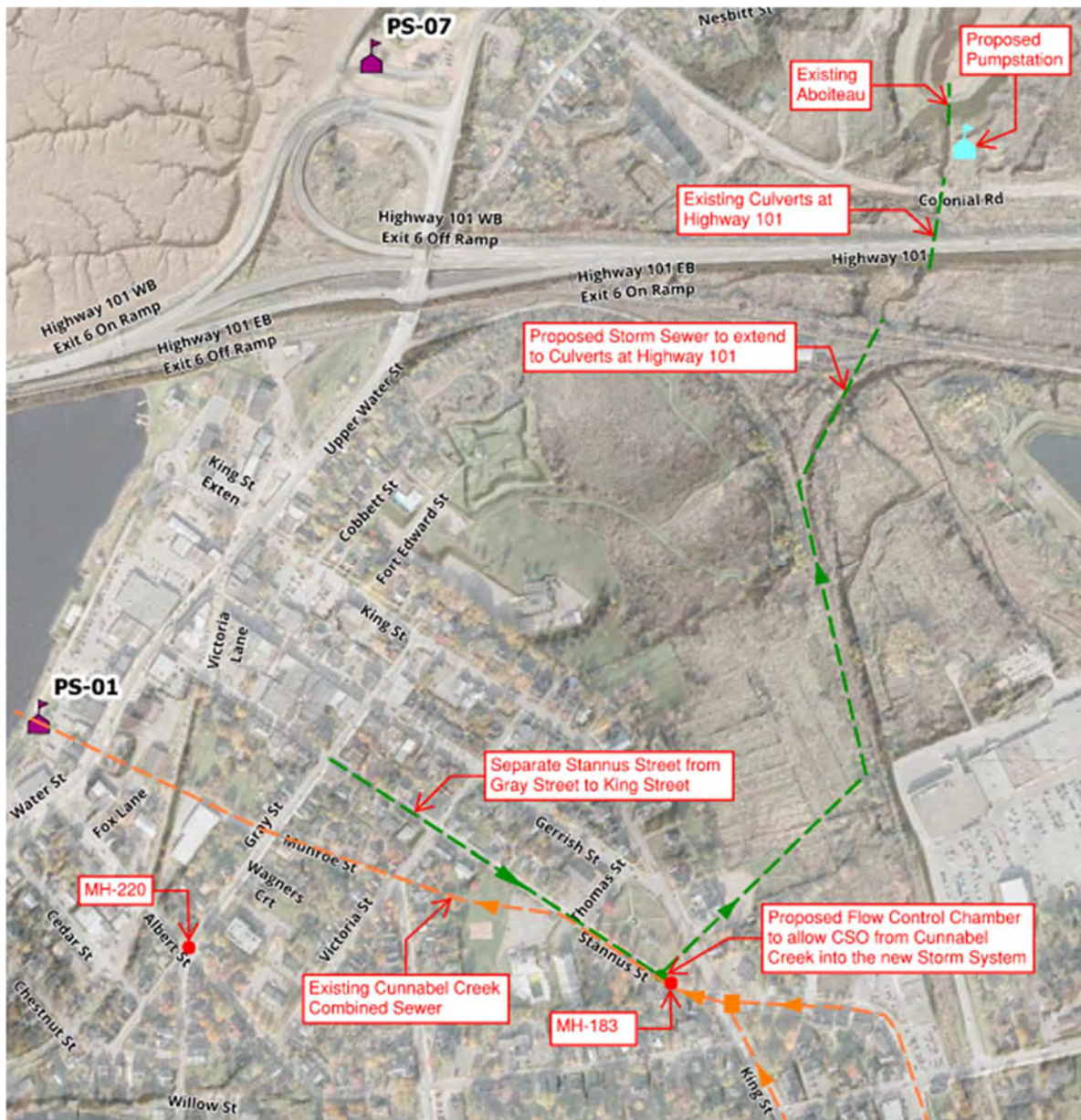
Figure 3.21: Proposed Layout Stannus Street Stormwater Connection to Tregothic Marsh
