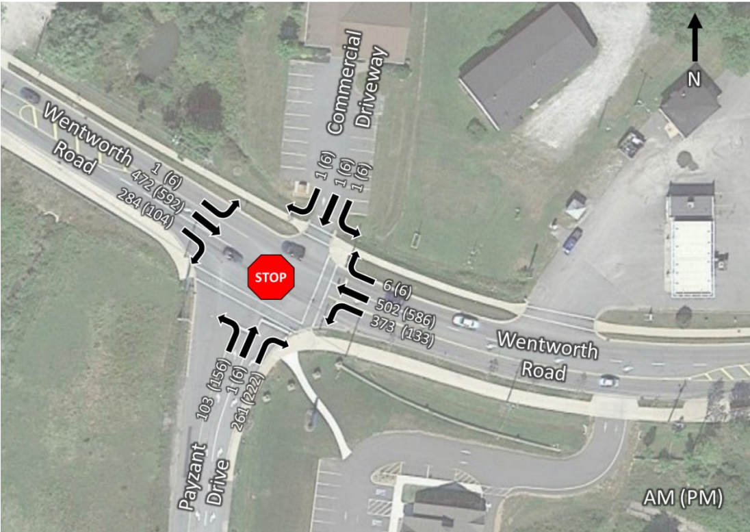
Figure 12 - 2033 future volumes for the AM and PM peak hours two-way stop controlled scenario
